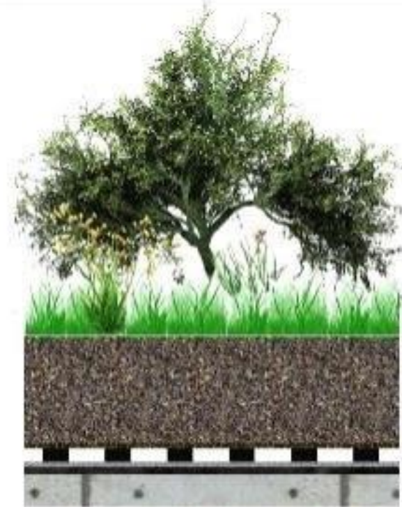
Intensive Green Roof
