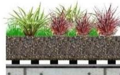
Semi-Intensive Green Roof
