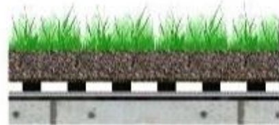
Extensive Green Roof
